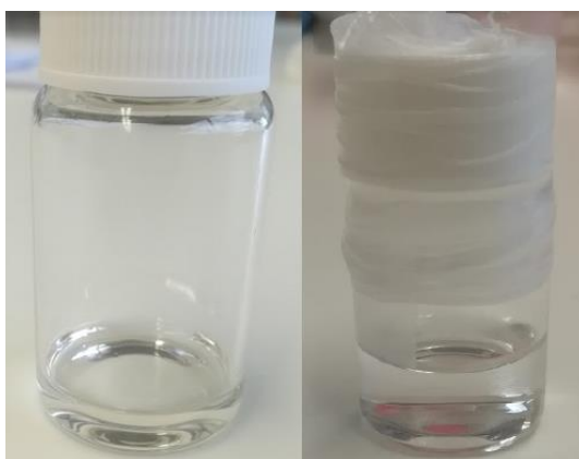
Figure 9 - OZ solubility tests in hydrophobic DES: C8:C12 DES on the left and C8:M DES on the right.
