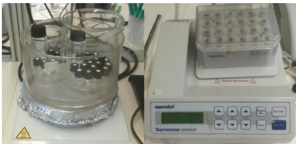
Figure 22 – Experimental set up to screen DES's ability to solubilize rice straw biomass.
